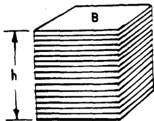
Figure 18-11.—Volume of a prism.
