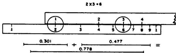
Figure 8-3.—Multiplication by use of the slide rule.
