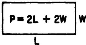
Figure 14-2.—Perimeter of a rectangle.
