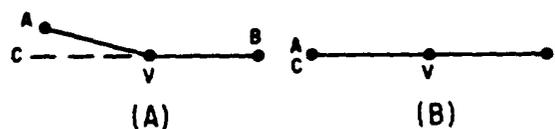
Figure 17-5.—(A) Large obtuse angle; (B) straight angle.
