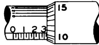
Figure 4B-Vernier micrometer.
