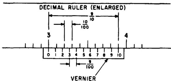
Figure 6-3.—Vernier scale.
