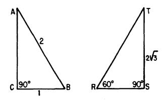
Figure 19-11.—Finding parts of 30°-60°-90° triangles.
