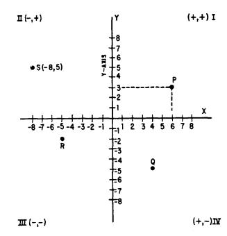
Figure 12-1.—Rectangular coordinate system.
