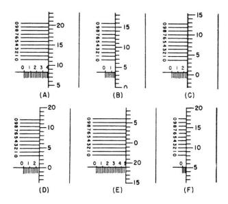
Figure 6-6.-Vernier micrometer settings.
