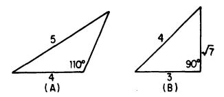
Figure 19-15.—Triangles which may be mistaken for 3-4-5 triangles.
