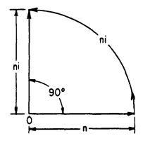
Figure 15-3.—Graphical multiplication by operator i.
