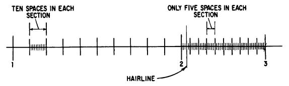
Figure 8-6.—Reading in the second division of a slide rule.
