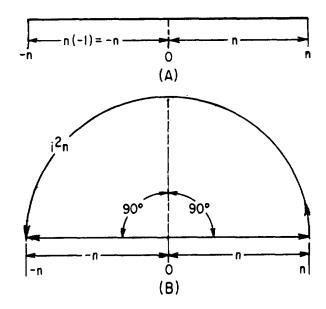
Figure 15-2.—Graphical multiplication by -1 and by operator i<sup>2</sup>.
