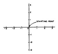
Figure 3-2.—Rectangular coordinate system.
