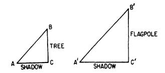
Figure 19-5.—Calculation of height by comparison of shadows.
