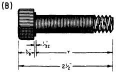
Figure 4-6.—Finding unknown dimensions by subtracting fractions.
