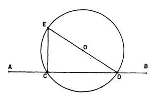
Figure 18-4.—Erecting a perpendicular at a point.
