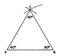
Figure 18-7.—Constructing 60° angles.
