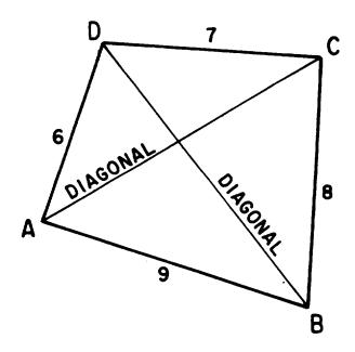
Figure 17-13.—Parts of a quadrilateral.
