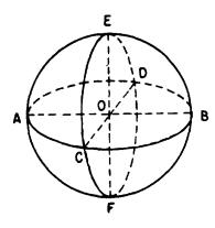
Figure 18-19.—Parts of a sphere.
