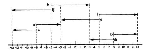
Figure 3-5.—Subtraction by use of the number line.
