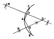
Figure 18-8.—Finding the center of a circle.
