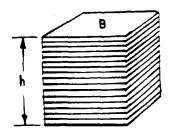
Figure 18-11.-Volume of a prism.
