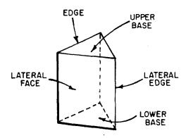
Figure 18-10.-Parts of a solid figure.
