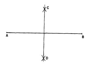
Figure 18-3.—Bisecting a line geometrically.
