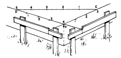
Figure 18-6.—Constructing a right angle by the 3-4-5 method.
