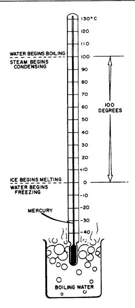
Figure 3-1.—Celsius (centigrade) temperature scale.
