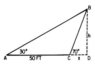
Figure 19-19.—Calculation of unknown quantities by means of oblique triangles.
