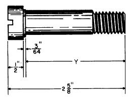
Figure 3B. -- Sketch of a machine bolt.
