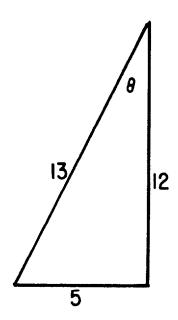
Figure 19-9.—Using trigonometric ratios to evaluate angles.
