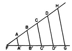
Figure 11A.--Dividing line FG into equal segments.
