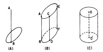
Figure 18-14.-(A) Line generating a cylinder;
