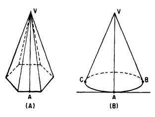
Figure 18-18.—(A) Slant height of a regular pyramid; (B) slant height of a right circular cone.
