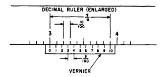
Figure 6-3.—Vernier scale.
