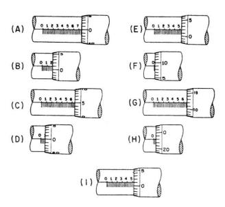
Figure 6-2.-Micrometer settings.
