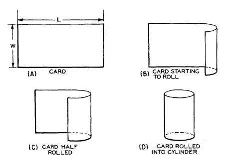
Figure 18-15.-Lateral area of a cylinder.
