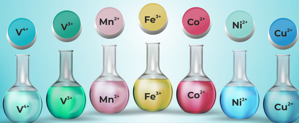
Colours of some of the first row transition metal ions in aqueous solutions. From left to right
